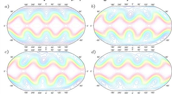
Figure 3. Free surface height after 12 days, contours from 8030 m to 10530 m, contour intervals of 100 m. Analytic solution (a), reference explicit solution with  $\Delta t = 900$  s (b), time and space regularized solutions (c and d, respectively), both with  $\Delta t = 2400$  s.
