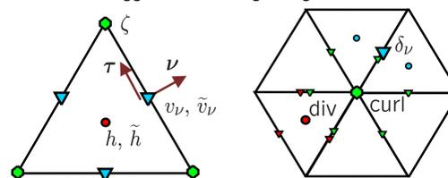
Figure 1. C-grid staggering, left, and stencils of the discrete operators  $\delta_{\tilde{v}}$  (blue), curl (green) and div (red), right.
