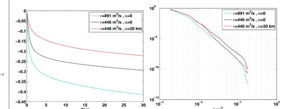
Figure 4. Decaying turbulence experiment: SW with viscosity  $\nu = 891 \text{ m}^2 \text{ s}^{-1}$  (blue), and  $\nu = 446 \text{ m}^2 \text{ s}^{-1}$  (black), and SW- $\alpha$  with  $\nu = 446 \text{ m}^2 \text{ s}^{-1}$  and  $\alpha = 20$  km (red). Left: energy dissipation; right: energy spectra at day 30. Results for SW- $\tau$ , not plotted, analogous to those of SW.
